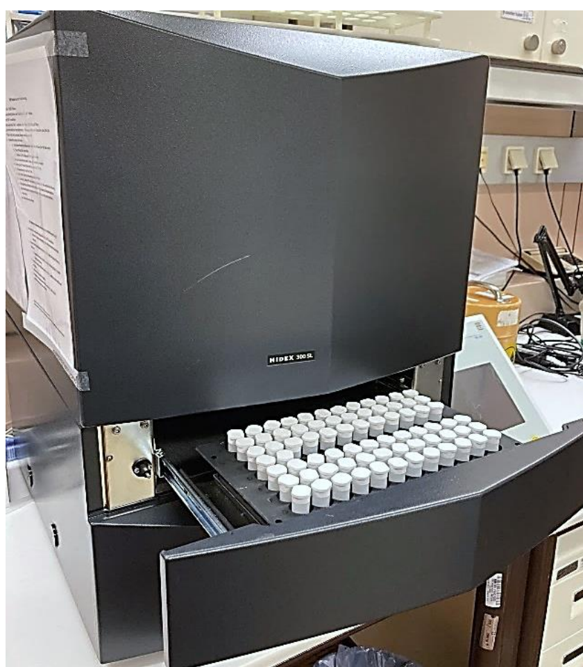
Figure 11: The Hidex 300 SL beta radiation counter is shown with the sample tubes already placed in the instrument. Medical University of Vienna, Nuclear Medicine Department.
