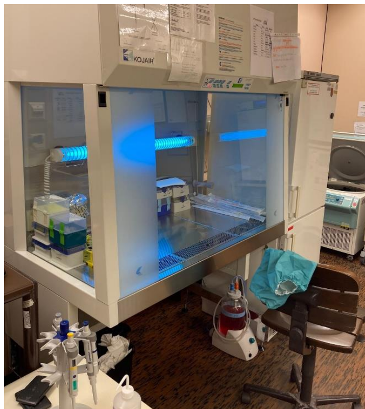
Figure 9: A picture of the laminar airflow sterile cabinet, the workplace in the cell culture lab. Medical University of Vienna, Nuclear Medicine Department.
