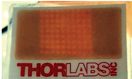
Figure 17: Picture of a 10 \times 10 trap array on a detector card, taken in the focal plane behind AODs. It was created by driving both AODs with ten different RF tones each separated by 1 MHz.
