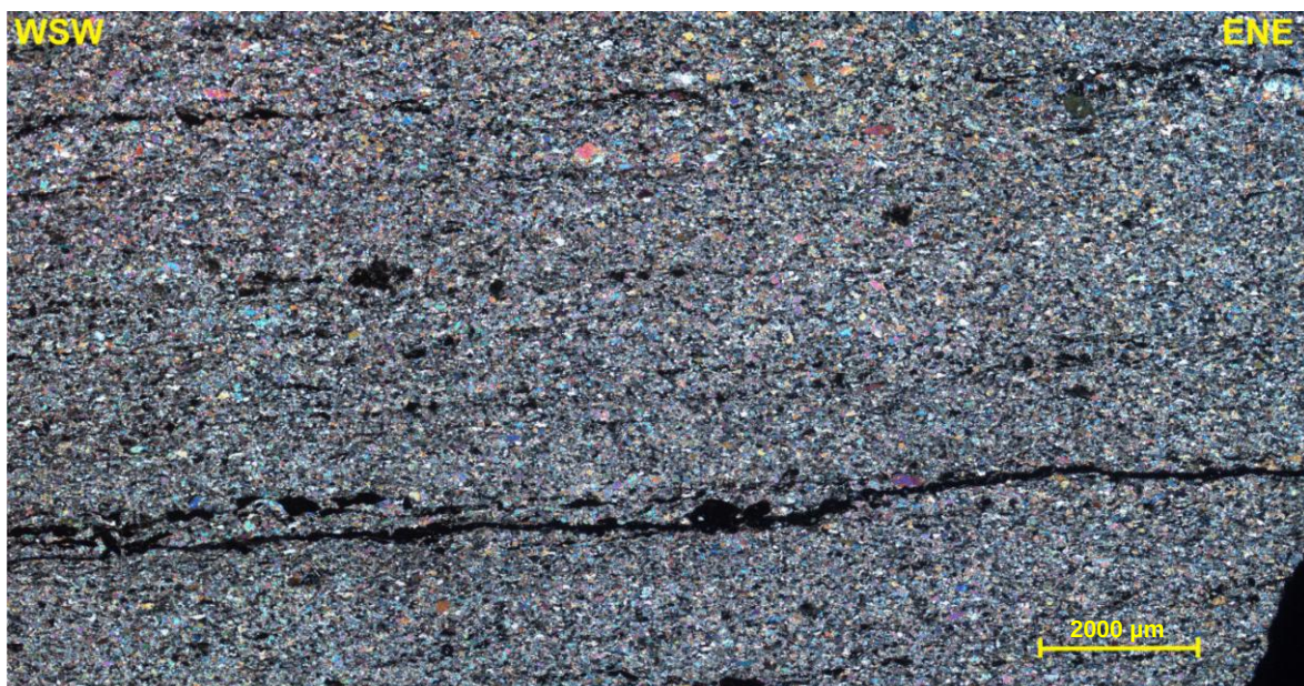
Fig. 5.38: Panoramic view of thin-section 12a, showing a recrystallised fabric of anhydrite (salt) mylonite. Grain sizes are relatively constant over the whole section, only few larger grains exist. Minor pressure solution cleavage is seen in this picture. The picture is taken under CPL.
