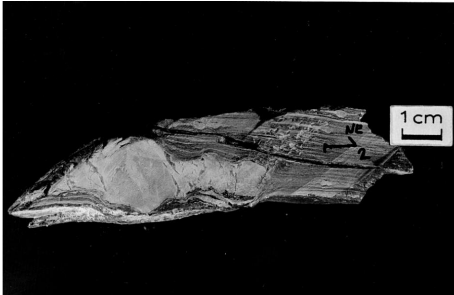
Fig. 5.35: Photo of sample 2, showing a clast of Hallstatt Limestone that is rotated and partly fractured in an anhydrite mylonite. The clast shows stairstepping that indicates top to NE direction of tectonic transport. Temperature conditions < 200°C
