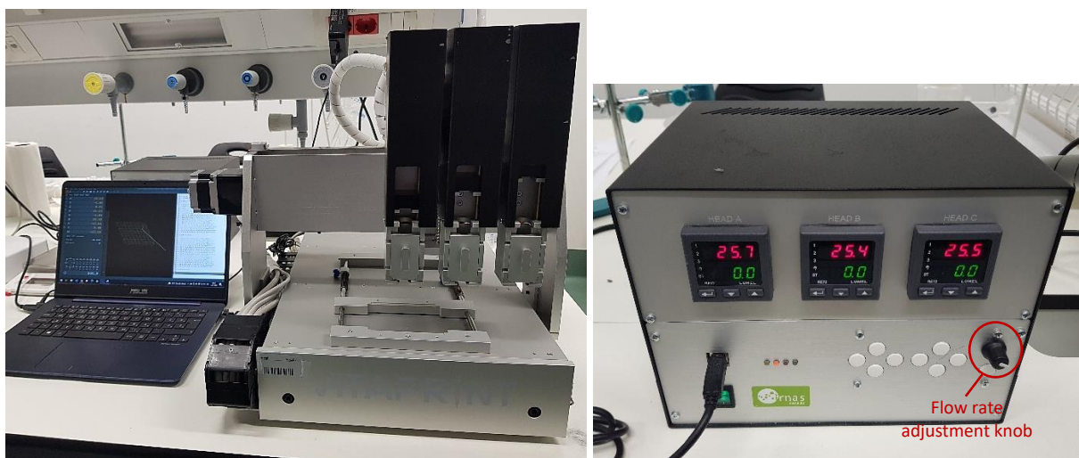
Figure 8. 3D printing device. Left: Vitaprint 3D printer connected to the computer; Right: the power generator with flow rate adjusting knob and temperature regulator for each printing head
