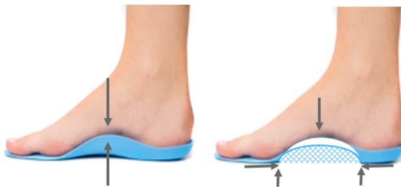
Figure 7.20. Compare the current shoe insole (left) to our novel design (right). The grey arrows represent the direction of the external force and reaction force
