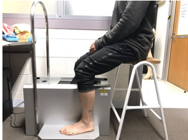
Figure 7.5. 3D foot image for insert design is scanned in non-weightbearing condition to keep the natural curve of the foot arch
