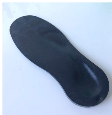
Figure 7.39. First prototype produced by OBJET Eden260VS using Tangoblackplus plus FLX980
