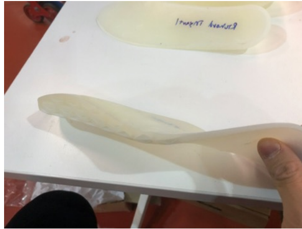
Figure 7.40. The second prototyping. The traditional solid and Honeycomb novel inserts were produced by Agilus 30
