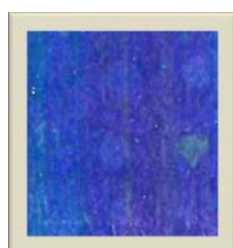
23 % PLGA 1% Desmodur Desmodur After 4 hours
