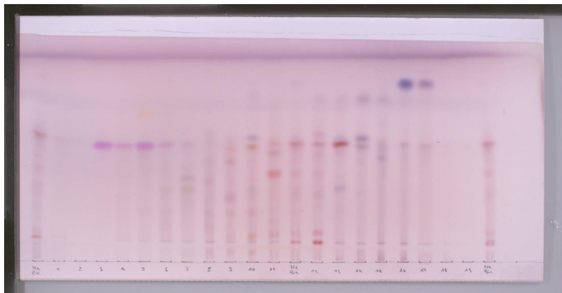
Figure A 11: FC01a (first Flash chromatography in this work); “NaBic” is the \text{NaHCO}_3 -extract as a standard (see chapter 4.2, p. 19)
