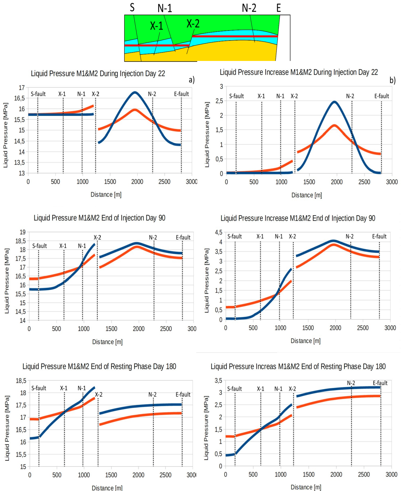
Fig. 16 Liquid pressure (a) and liquid pressure increase (b) compared between model M1(blue) & M2 low (red); from top to bottom: a sketch of the storage structure and the line where liquid pressure was exported, liquid pressure and liquid pressure increase during injection (day 22), at the end of injection (day 90) & at the end of the resting phase (day 180). Note that fault X-2 marks a strong offset in the reservoir; therefore, liquid pressure is relatively high in the SW of X-2
