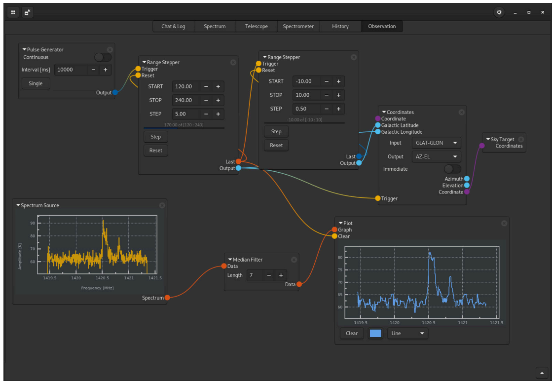
Figure 4.1: A custom grid observation programme of a section of the galactic plane. A pulse generator instructs the range steppers to generate the coordinate outputs for a grid scan between galactic latitudes \pm 10^\circ and longitudes 120^\circ to 240^\circ , which are converted to the telescope's reference system and then sent to the instrument. A source node for spectral data provides output, which is filtered and the result is displayed. Note that this figure shows only a subset of planned functional nodes.
