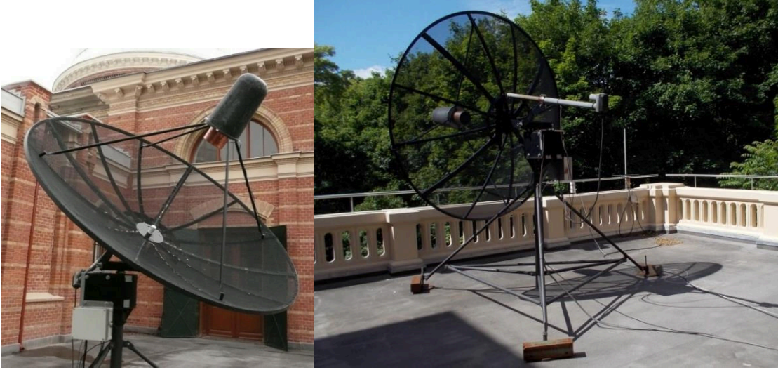
Figure 2.15: The Small Radio Telescope as operated by the Department of Astrophysics at the Vienna University Observatory. (Photos courtesy of H. Chmela)
