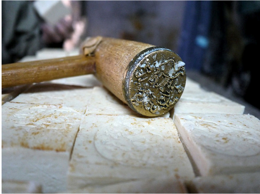
Figure 4.3.: xatm or mdaqqa for stamping the factory logo onto the soap. Courtesy of Alnaameh Nabulsi soap company.
