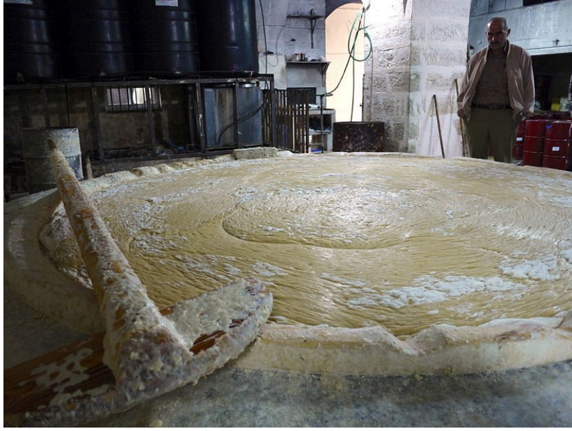
Figure 4.1.: ḥalle for cooking soap. Courtesy of Alnaameh Nabulsi soap company. ( annaṣāma )
