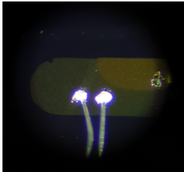
Figure 3.17: Damage done to the gold pads by the wirebonder.
