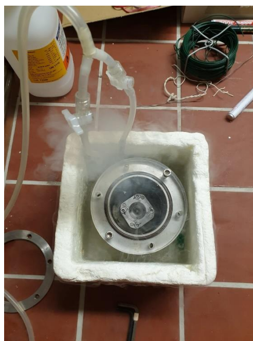
Figure 3: Flooding of the DAC with liquid argon
