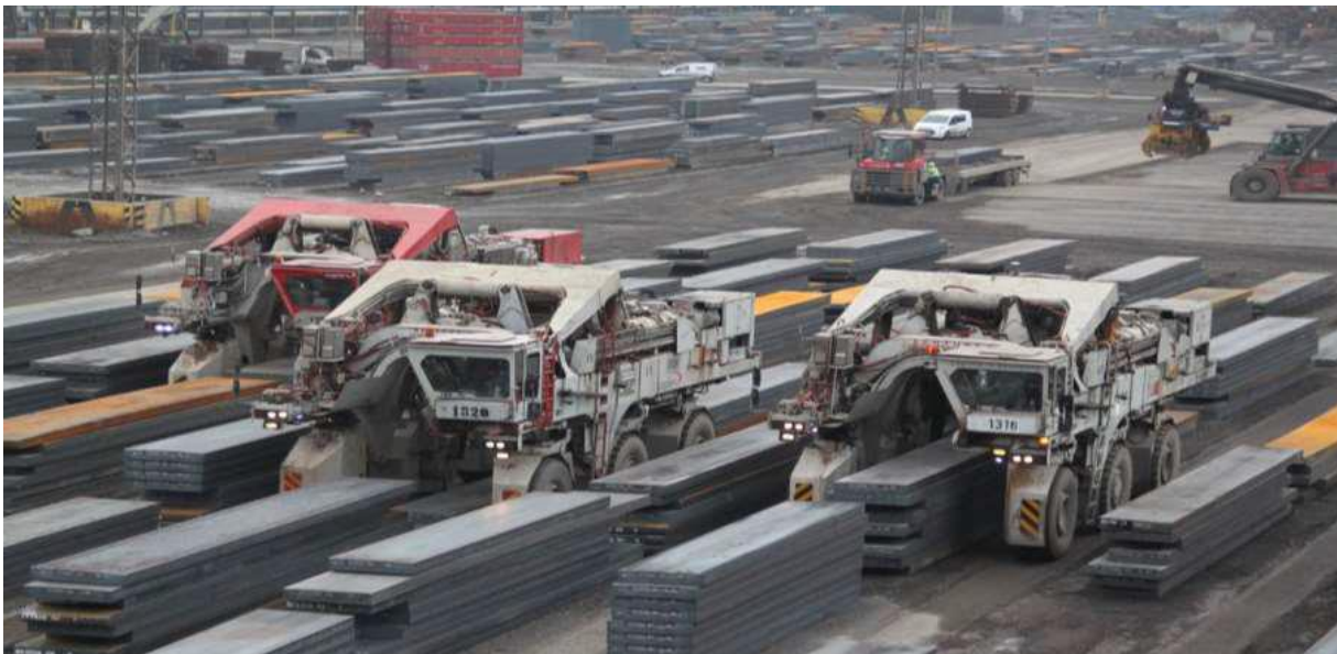
Figure 11. Straddle carriers moving over rows of slab stacks. (source: voestalpine Stahl GmbH)
