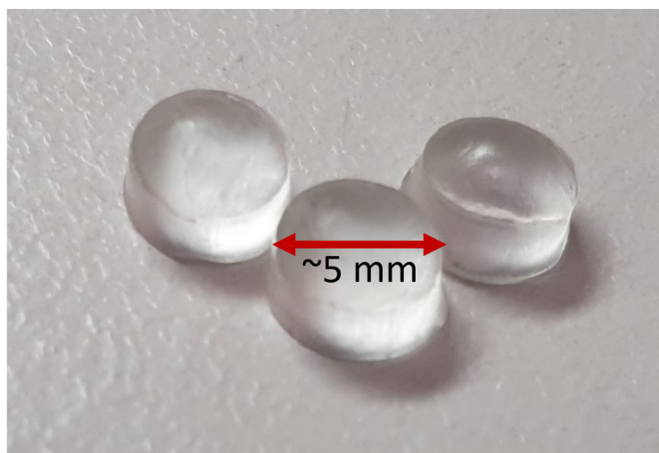
Figure 4: PVC MP pellets with a diameter of \sim 5 mm.
