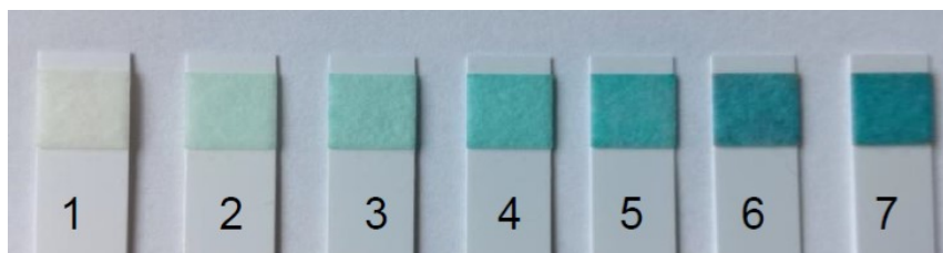
Figure 30: Calibration of glucose test strips using standard series of glucose.
