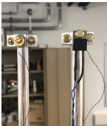
(b) Aluminium clasp mounted to the ends of the rods. Each holds one temperature sensor (left) and one heating resistor (right).
