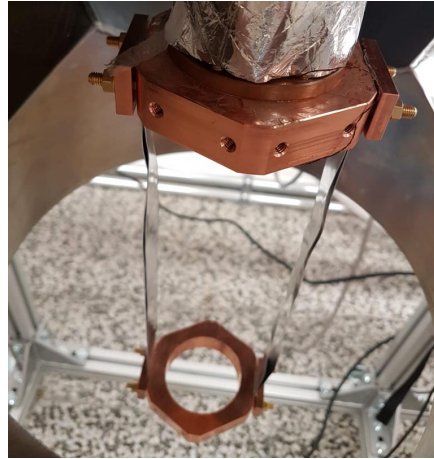
Figure 27: Testing setup using indium as a thermal contact agent.
