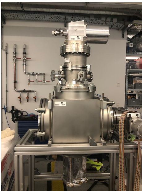
(b) Photo taken of the SIDDHARTA-2 target cell testing chamber.
