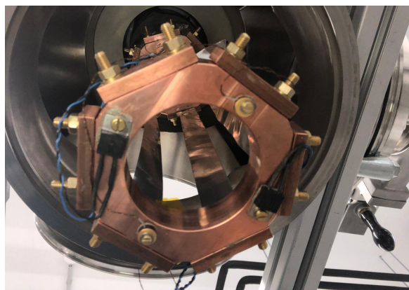
(c) Bottom copper holder including Diodes 1 and 2 and Resistors 1 and 2.
