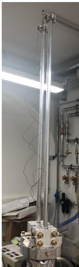
(a) Mounting of the 5N aluminium bars. They are attached to the sample holder of the cold head via two aluminium flanges (bottom).
