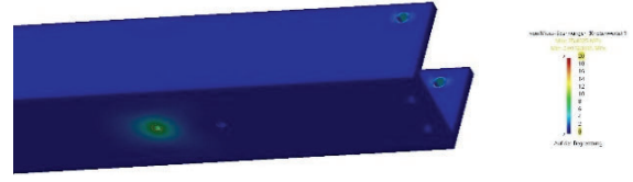
Figure 4: Von Mises stress on polyamid U-Profile (Stummer, 2016).
