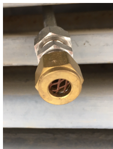
Figure 3.7: Inlet for the Vienna urban aerosol
