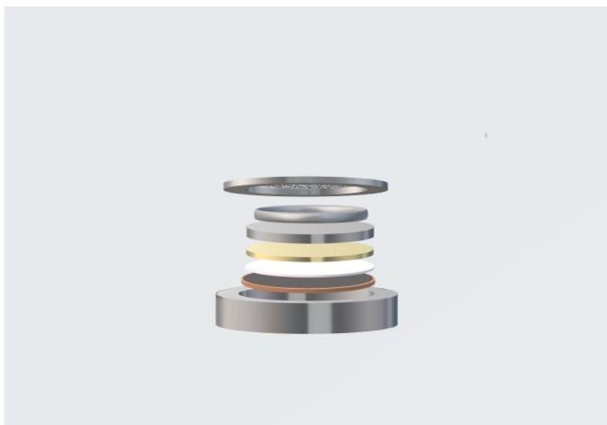
Figure 13: Illustration of a schematic coin cell. From bottom to top: bottom cap, Cu current collector coated with \text{SnS}_2 active material (cathode), separator, Li metal (anode), spacer, spring, top cap. Reproduced with permission from Albina Glibo.
