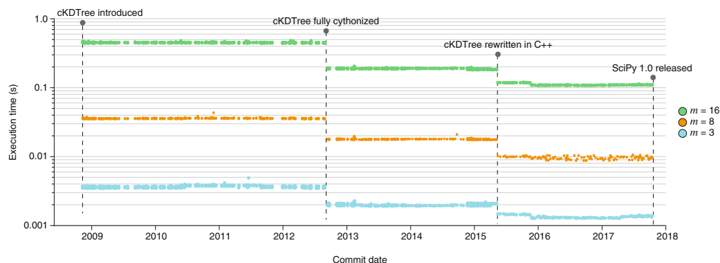
Fig. 3 | Results of the scipy.spatial.cKDTree.query benchmark from the introduction of cKDTree to the release of SciPy 1.0. The benchmark generates a k -d tree from uniformly distributed points in an m -dimensional unit hypercube, then finds the nearest (Euclidean) neighbor in the tree for each of 1,000 query points. Each marker in the figure indicates the execution time of the benchmark for a commit in the master branch of SciPy.
