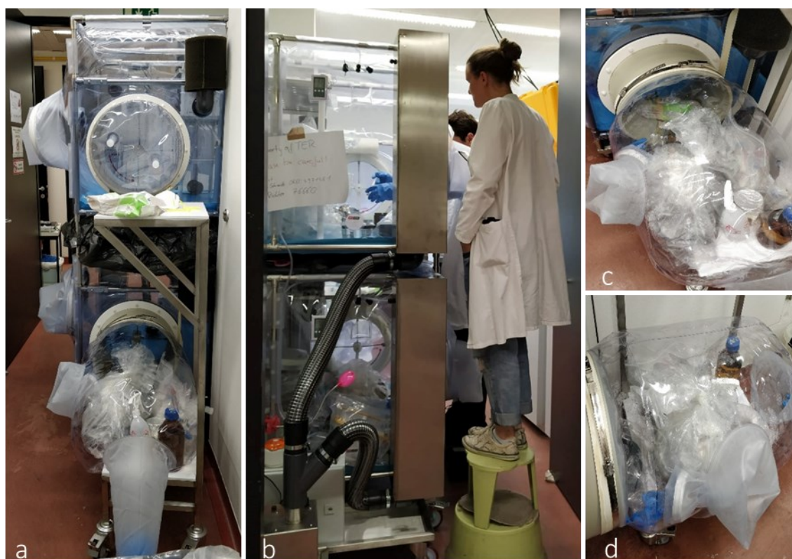
Figure 1 The isolator (right side and left side; a + b ) providing a sterile environment within its lower and upper chamber by filtering incoming air via a HEPA (high efficiency particulate air) filter. Both chambers have a round-shaped port system to which a smaller chamber ( c + d ) can be attached to bring equipment in after being disinfected. Picture credit b : Carolina Urbina Malo, MSc.
