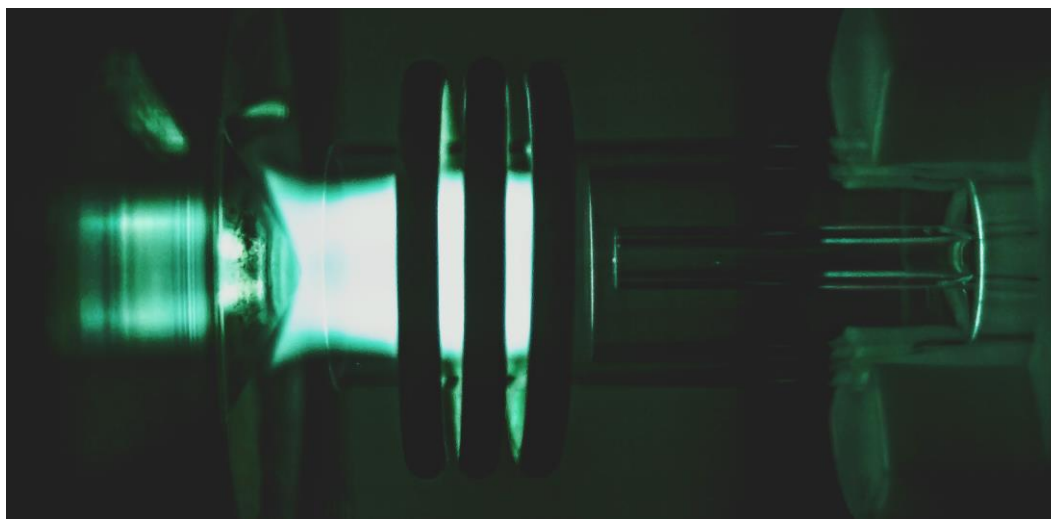
Figure 6: Close-up of inductively coupled plasma in an ICP-MS instrument
