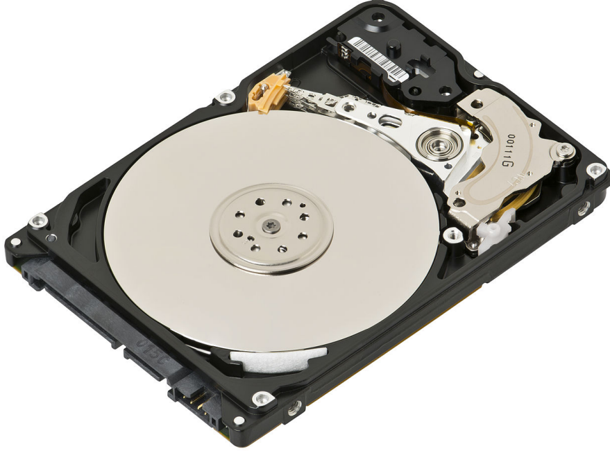
Figure 1.1: Opened hard disk drive showing the platter and the actuator arm with the write and read head on the tip (orange area). Picture taken from [7].
