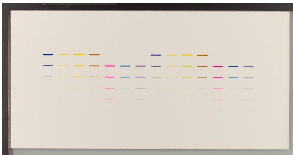
Figure 17. HPTLC sampling of the tracer dyes to determine the optimal concentration
