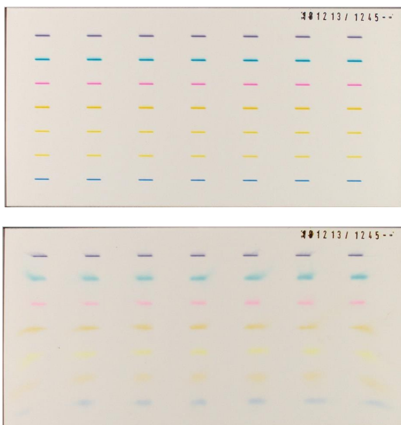
Figure 19. Top: HPTLC sampling of the tracer dyes to determine the dispersion of the dyes. Bottom: After blotting the same silica plate.
