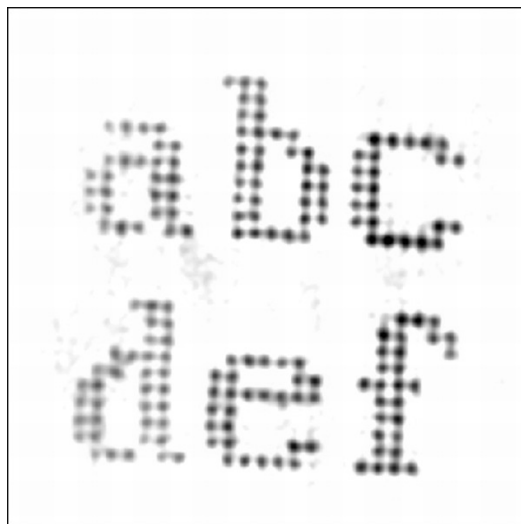
(d) Image of the specimen as reconstructed from the diffraction pattern by an iterative algorithm.
