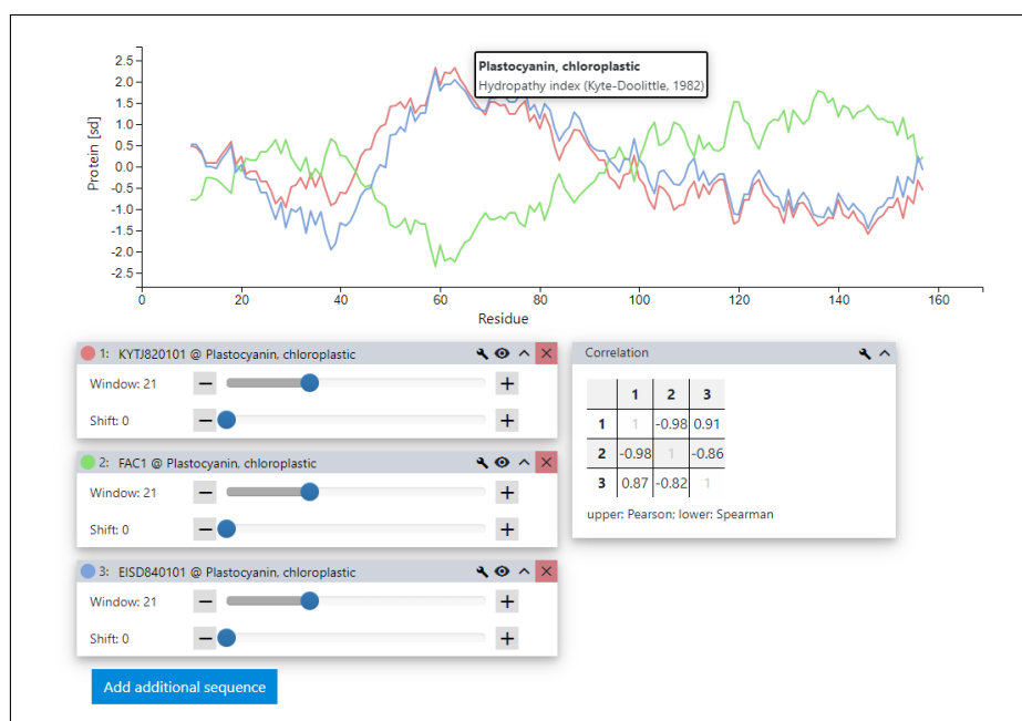
Figure 2: Example of the VOLPES interface The same protein sequence as in the previous examples was used (Plastocyanin from Pisum sativum ), but since VOLPES supports parallel analysis of multiple profiles, three different protein hydropathy measures were used at the same time -the Kyte & Doolittle scale, as used in the previous examples, the Eisenberg consensus hydrophobicity scale and Factor 1 from Atchley and coworkers[44]. To make comparisons between different properties easier, VOLPES allows one to rescale profiles by their standard deviation as used here. Details about a profile can be seen by simply hovering the mouse over a profile, while correlation coefficients, capturing the similarity between different profiles, can be accessed in the table on the bottom left. A new box in the interface has been created for each profile. Importantly, all parameters, including the sequence, the scale used, the smoothing window and the shift relative to other sequences, can be changed interactively without having to exit the current state of analysis.
