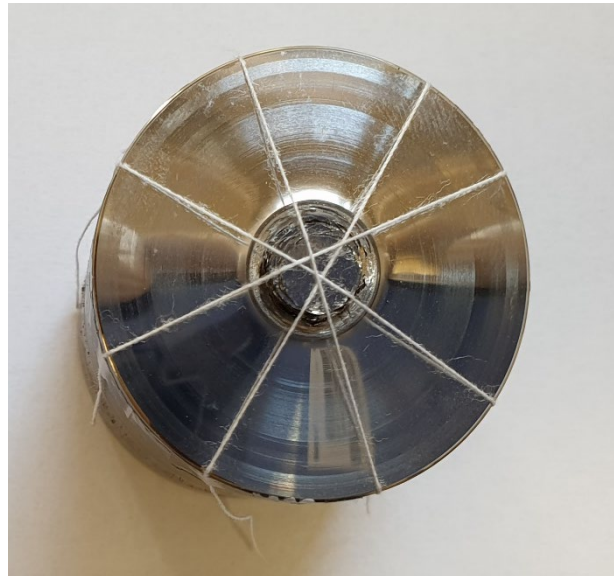
Figure 3.3: Sample preparation of FINEMET Amorphous material.
