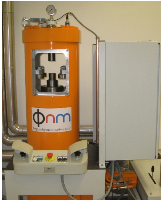
Figure 3.1: Photograph of High-Pressure Torsion (HPT) equipment available with the Research Group Physics of Nanostructured Materials at the Faculty of Physics, University of Vienna.
