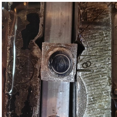
Figure 3.4: Various steps in the formation of ring samples for magnetic measurements through spark erosion machine.
