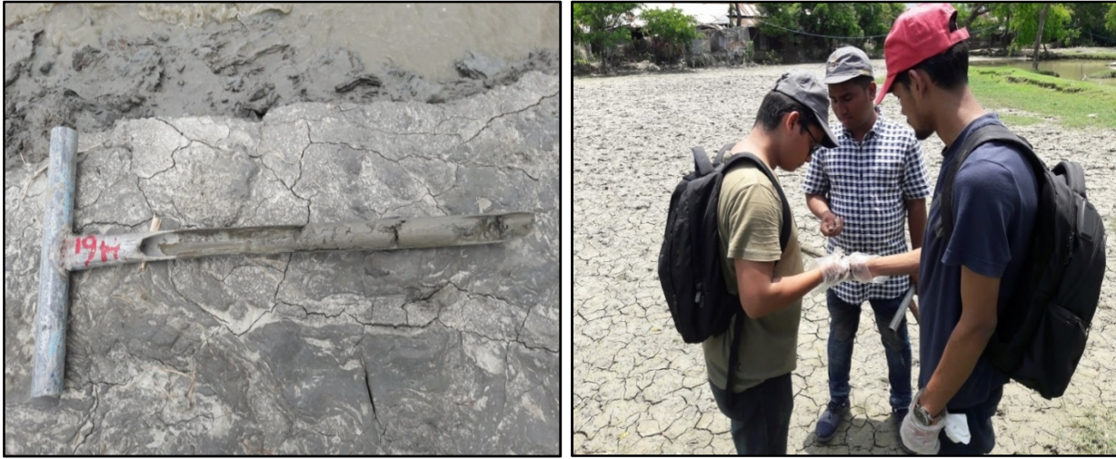
Figure 3.4: Collection of Soil sample using bore-hole and determining the sediment texture in the field.
