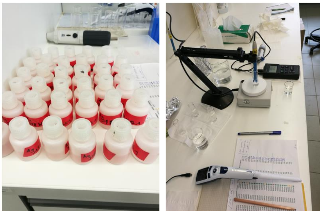
Fig. 3.6: Photographs of anion samples and titration setup for \text{HCO}_3^- calculation at the UFZ in Halle. (Photographs: Heinzle 2018).
