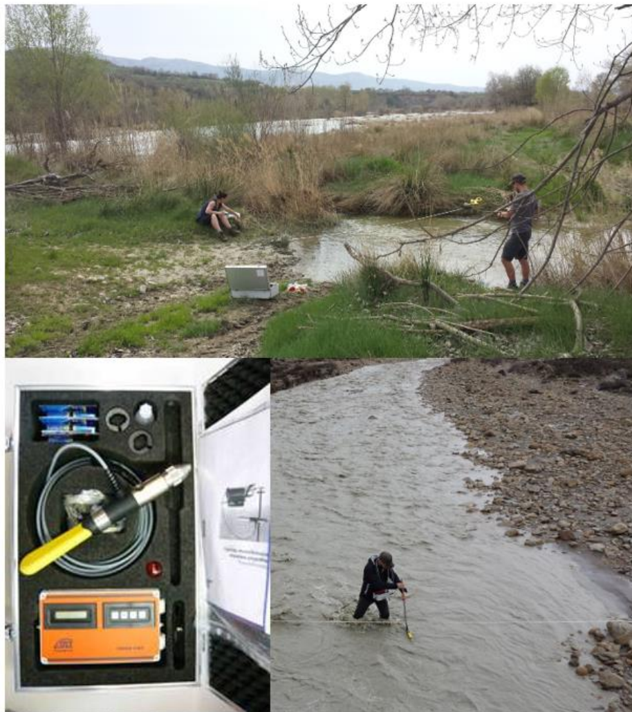
Fig. 3.4: River discharge measurements with subsections. Top: Tributary sampling (w33) before entering the main Isábena stream. Bottom right: Tributary in marl area (w7). Bottom left: OTT Nautilus C2000. (Photographs by: Konzett/Heinzle).
