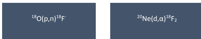
Figure 5. Nuclear reactions for the production of fluorine-18
