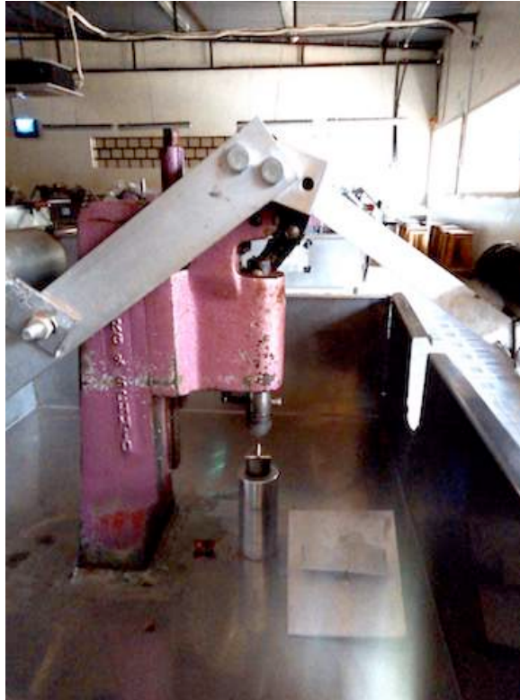
Figure 14: Hand-cracking machine for macadamia nuts, developed by Limbua; Source: Photographed by the author at Limbua factory 2018
