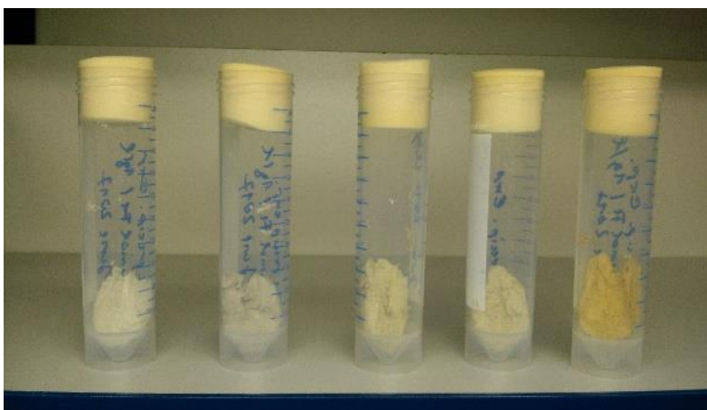
Figure 1.) Preconditioning of fibers and the resulting change in colors. From left to right: DFOB-altered fibers with 0, 3 and 30 \mu\text{mol g}^{-1} Fe, respectively, blank-altered fibers with 0 \mu\text{mol g}^{-1} Fe and DFOB-altered fibers with 300 \mu\text{mol g}^{-1} Fe.
