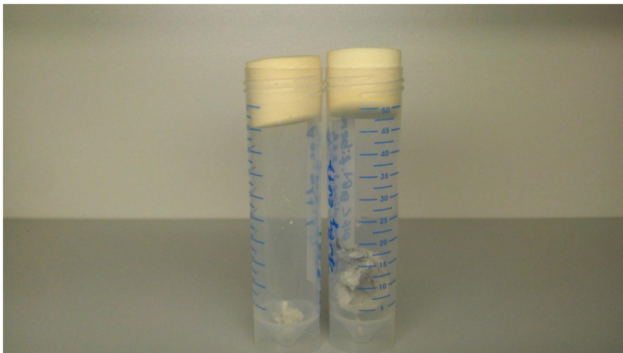
SI-Figure 2.) Color of re-oxidized ascorbate altered fibers. While ascorbate altered fibers had a pale-pinkish color, the color of re-oxidized ascorbate altered fibers (in the right tube) was greyish to brownish. As a comparison, the blank altered fibers (left tube) with a brownish color were added.
