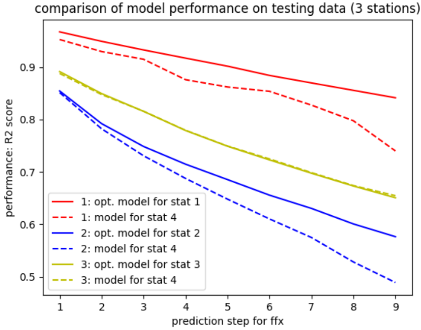
Figure 4.6: Models optimized for individual stations (1-3) versus models optimized for a fourth station (gust prediction).
