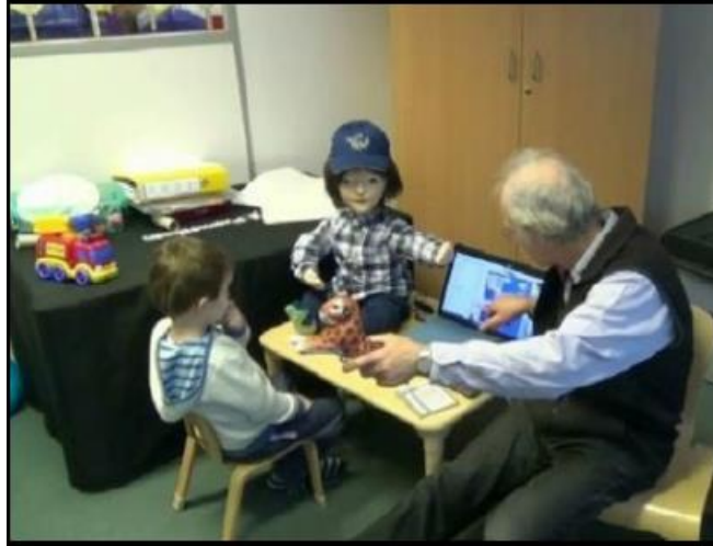
Figure 19 - The investigator showing the child participant in US1 what Kaspar "sees" through its cameras. Reproduced from D6.1 Use Case 3 Specification and Initial Report on Multi Party Child-Robot Collaboration and Learning, by Dautenhahn et al., 2017, p.32, Fig.3.(left). In the public domain.
