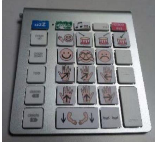
Figure 17 - The wireless keypad controlling Kaspar, the social robot to perform certain activities. Reproduced from D6.1 Use Case 3 Specification and Initial Report on Multi Party Child-Robot Collaboration and Learning, by Dautenhahn et al., 2017, p.31, Fig.2. In the public domain.
