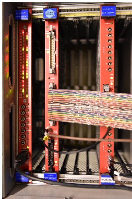
Figure 18: DAQ system used at the SMI consisting of a V1718 VME crate, a V785 ADC and a V1290 TDC by CAEN.
