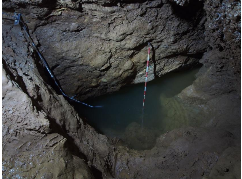
Figure 10: Left: Rock sample of the host rock from EISE. Photograph shows about 15x25 cm; right: Thermal spring with stick gauge and data logger.
