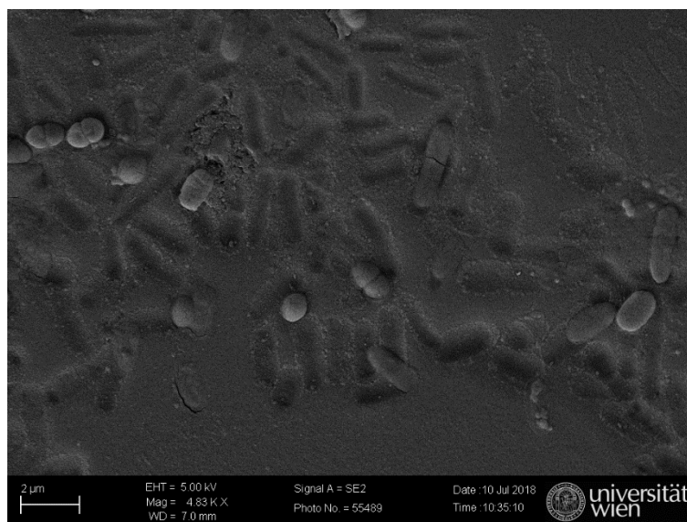
Figure 35: SEM image of E. coli located in the cavities of the BIP-beads; results were obtained from the rebinding experiment in an E. coli water suspension
