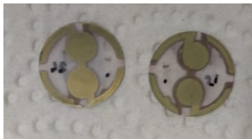
Figure 15: QCMs with screen-printed electrodes; on the left QCM, the top side is captured; on the right QCM, the bottom side is captured
