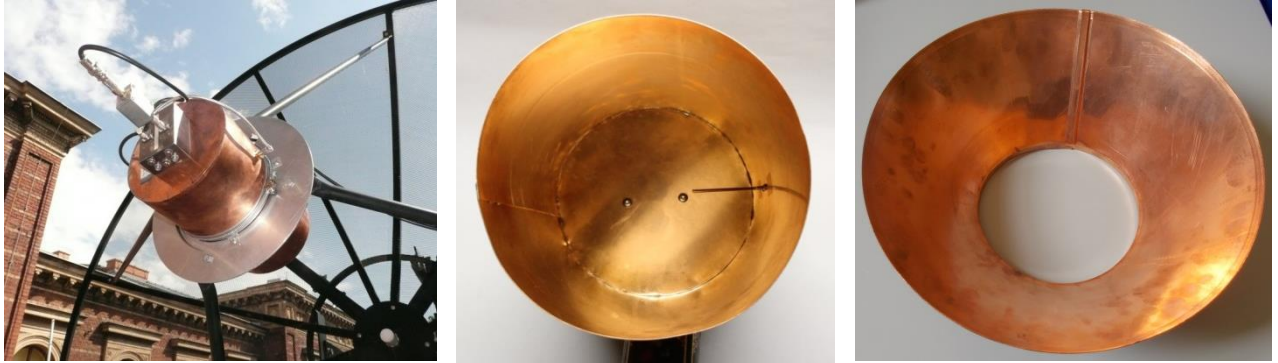
Figure 9: Primary focus assembly with original amplifier mounted at the SRT (left), inside view of the can antenna (middle) and attachable funnel for the can antenna (right)
