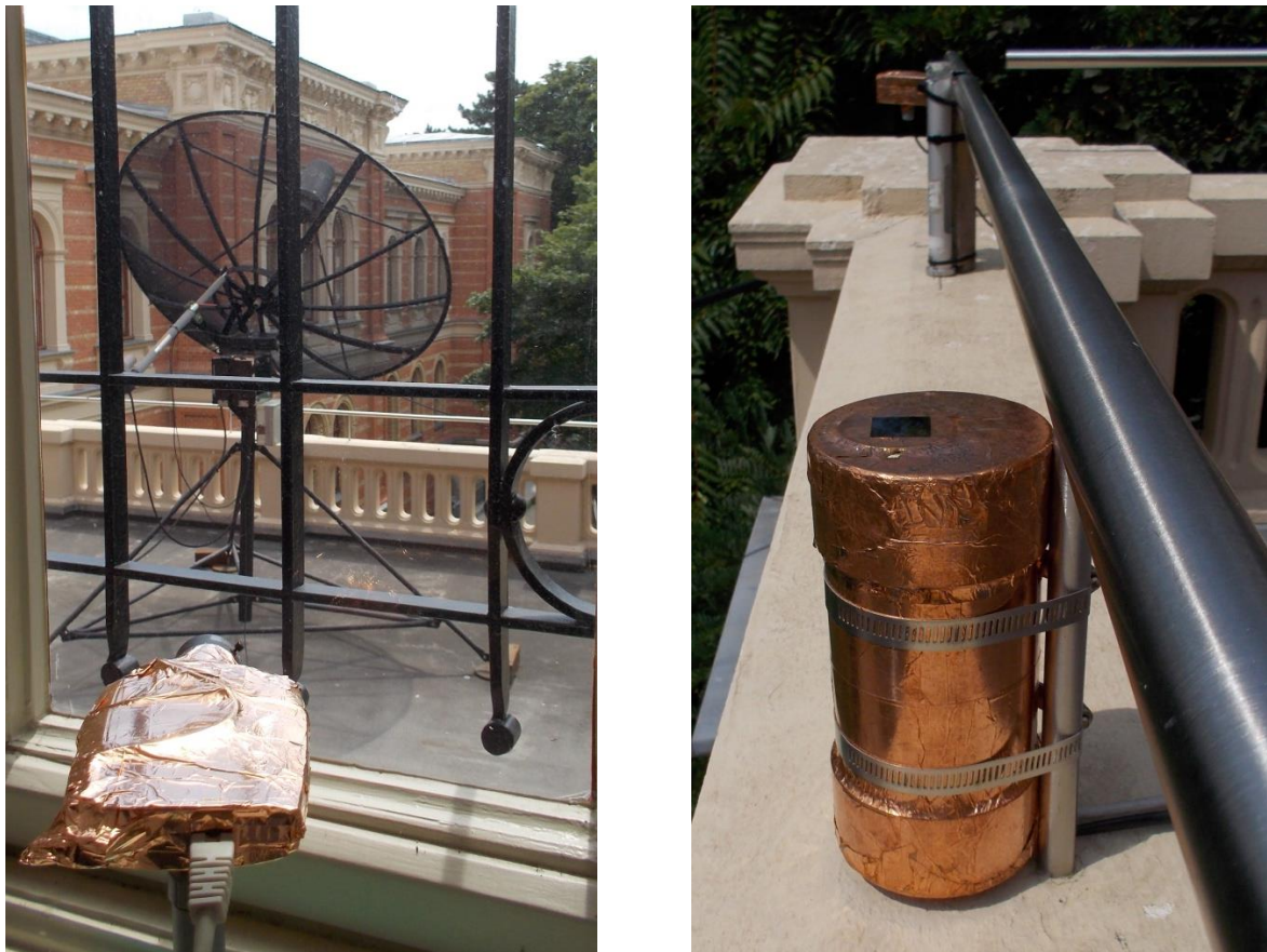
Figure 74: Shielded webcam next to the SRT (left) and shielded sky quality meters (right). SQM 1 in the foreground and SQM 2 in the background.
