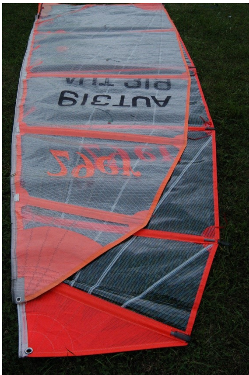
Fig. 50 Different 29er sail shapes. On the bottom the prototype squaretop, on top the standard pin head. (Author)
