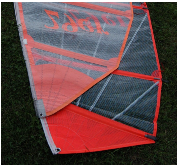
Fig. 30 The slightly larger prototype rig sail underneath the standard main sail. (Author) The size of the square top appears larger as there is no curvature of the mast
