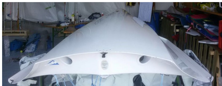
Fig. 15 Picture of a 29er Hull with the flat but wide transom and a very pointy and narrow bow. (Author)
