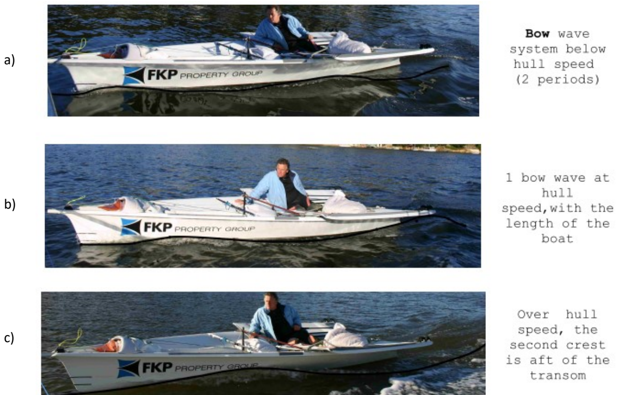
Fig. 16 Towing test of a 49er hull at below (a), exactly at (b) and over (c) hull speed. The black line along the wave patterns indicate the wave systems at various speeds. (13)
