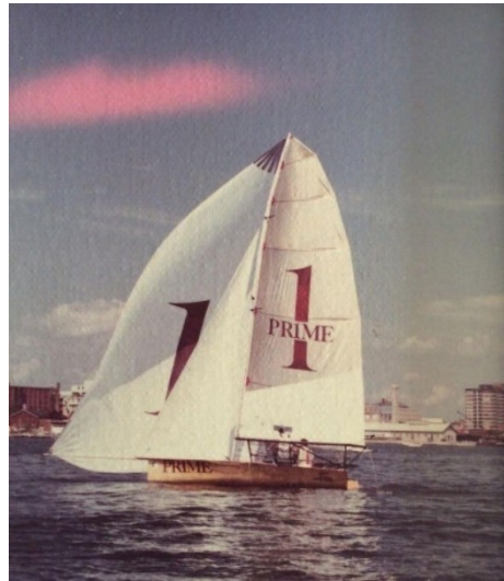
Fig. 49 Julian Bethwait's Prime I a two handed 18 Footer) with a "pin head Mainsail" (Author)
