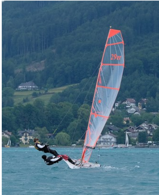
Fig. 11 A 29er sailing skiff in a gust. The twist in the sail can be seen as the upper end of the leech is much further to leeward than the part fixed to the boom. (Author)
