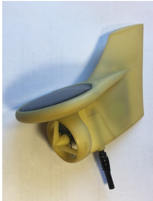
Fig. 23 The wind measuring system „IQ“ developed by Julian Bethwaite. (Author)
