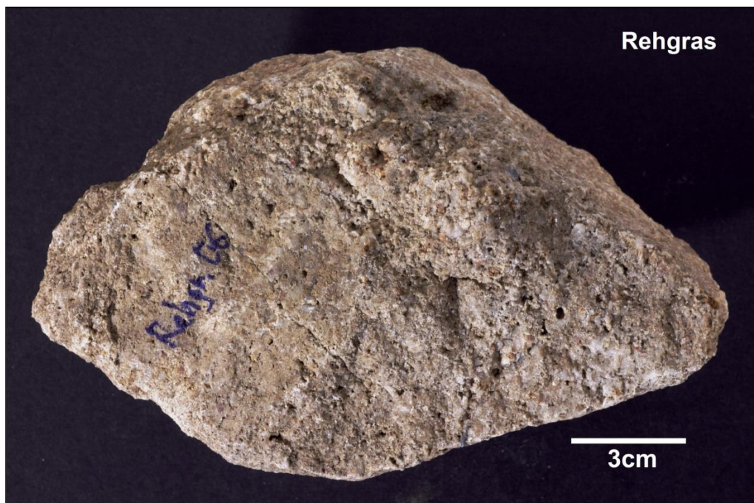
Fig.8 Dislodged slice of Groisbach: fine grained, strongly weathered, appears good sorted, grey-brownish color; dislodged slice of Rehgras: currently regarded as Keuper sandstone; coarse grained, poorly sorted rock with a greyish-brown crust;
