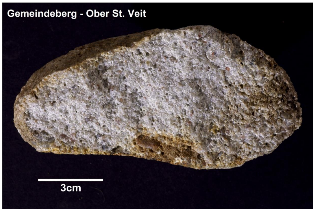
Fig.4 Samples, which are currently regarded as Keuper sandstones of the St. Veit Klippenzone, LT31/1200m (previous page): coarse grained and poorly sorted; note the large, colored quartz grains; LT31/1215m: a medium grained, overall better sorted sample indicates a range of medium to coarse grained composition for the Keuper sandstones of the Lainz tunnel section; Ober St. Veit: coarse grained; poorly sorted; samples from the Gemeindeberg are mainly strongly weathered
