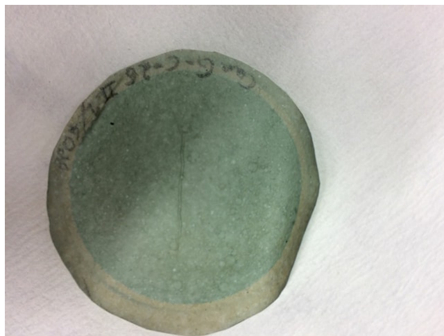
Figure 34: CSG nanopaper after filtration of a copper nitrate solution.
