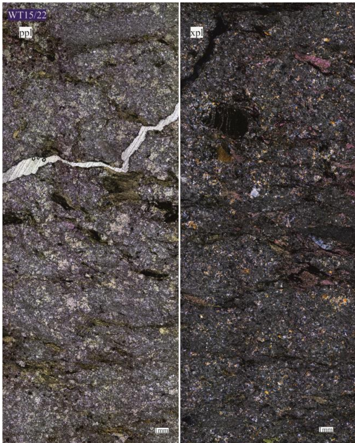
Figure 26: Overview of the thin section of sample WT15/22 of fine-grained sandstone part of lithofacies 10 shown with parallel polarizers (ppl) on the left and crossed polarizers (xpl) on the right side..
