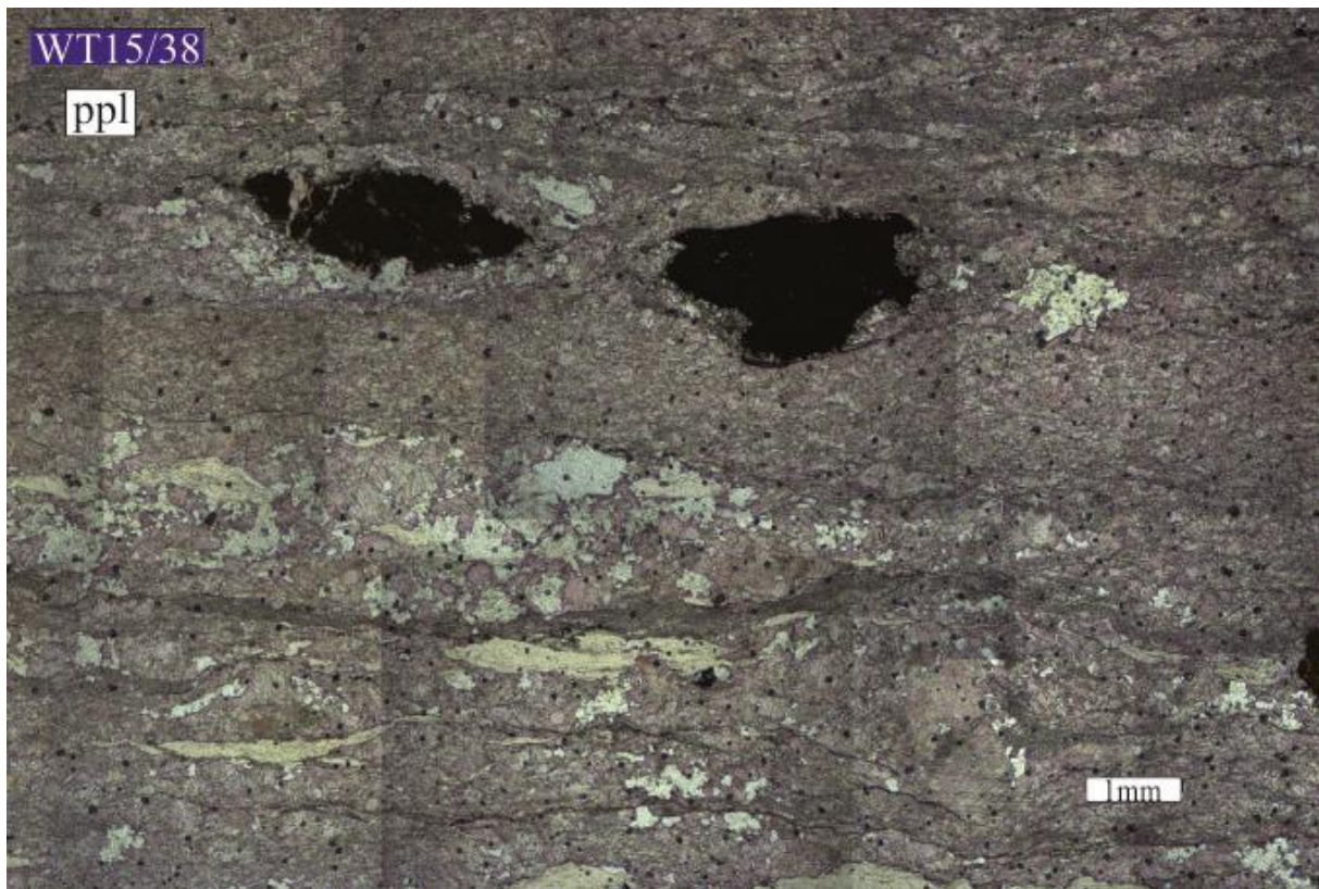
Figure 30: Overview of the thin section of sample WT15/38 of lithofacies 13 shown with parallel polarizers (ppl). Noteworthy are the micritic dolomite clasts further explained in chapter “thin sections”.
