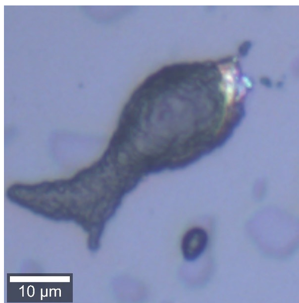
Figure 4.24: E. coli cells embedded in a DVB/Styrene matrix; after the immersion of the E. coli imprinted polymer sheet in E. coli solution, different spectral components were expected.
