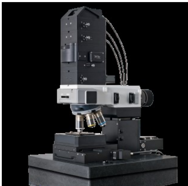
Figure 2.8: WITec Alpha 300R Raman microscope; a confocal microscope is coupled to a Raman spectrometer. The laser beam is directly focused through the microscope objective. The scattered light passes through the spectrometer and is detected by a cooled CCD camera.
