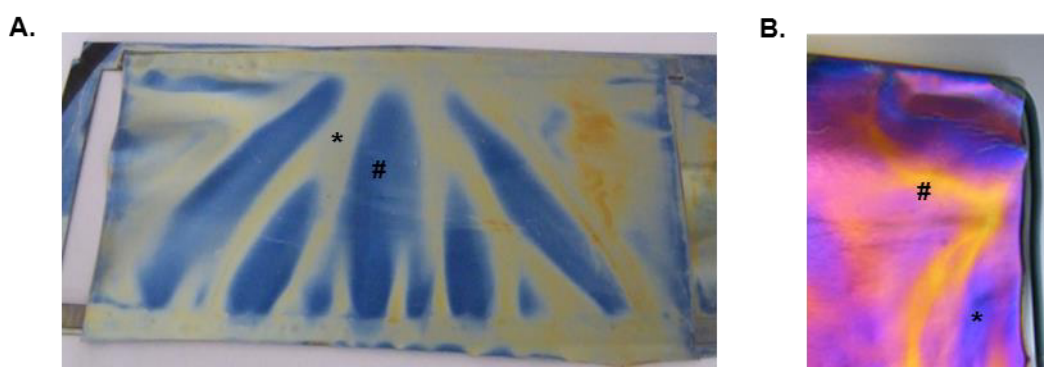
Figure 25 | Flow defects on corrugated TPU REA films A) TPU RHS film The prominent areas (“hills”) exhibited a yellow resonance color indicating a locally thicker interlayer (= \text{SiO}_2 distance layer + PEM) (*... hills, #... valleys). B) TPU REA film without (w/o) humidity sensor layer The prominent areas of this sample also carried a thicker \text{SiO}_2 distance layer appearing in blue-violet on a yellow-pink background (*... hills, #... valleys).
