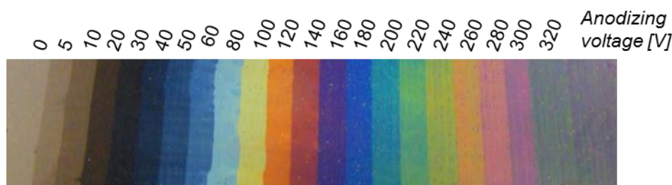
Figure 35 | Aluminum-based REA color palette with Pd cluster layer
