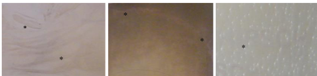
Figure 56 | Defects in \text{TiO}_2 coatings Thin layers of \text{TiO}_2 were deposited on the mirror layer of the depicted RHS films by precipitation from solution. The films exhibited irregularities (marked by asterisks), which either resembled marbling (left and middle) or small granular, rather homogeneously distributed aggregates.
