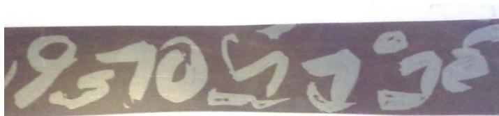
Figure 58 | Non-sensor REA film patterned by masking with Eudragit/ ethyl cellulose solution
