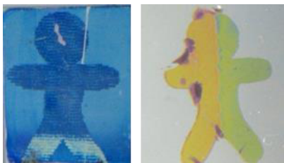
Figure 55 | Multicolored patterns on REA films Two-colored patterns were generated on REA films by direct patterning of \text{SiO}_2 layers using nitrocellulose masks. Metal clusters were either deposited homogeneously over the whole REA film surface (left) or only in the shape of a stick figure (right). In the second case surrounding area was protected by adhesive tape. Therefore the background is non-colored but silvery metallic.
