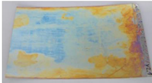
Figure 30 | First test of Endless Band Coater A) Non-sensor REA coating B) Complete RHS coating
