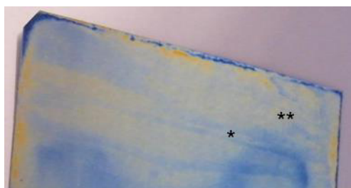
Figure 21 | Linear defects on RHS film The depicted RHS film with blue base color exhibited yellow wavy lines (*) and linear patches (**) at both short ends.
