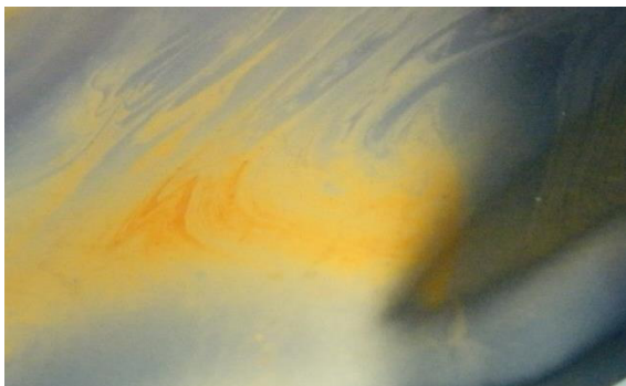
Figure 23 | Marbling defects in REA humidity sensor coating
