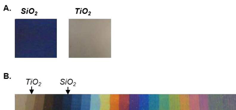
Figure 57 | Comparison of \text{SiO}_2 and \text{TiO}_2 deposition protocols A) REA films with Al mirror layer, Pd metal cluster layer and either \text{SiO}_2 (left) or \text{TiO}_2 (right) distance layer B) The color of the two REA films is indicated above the depicted Al-based REA color standard
