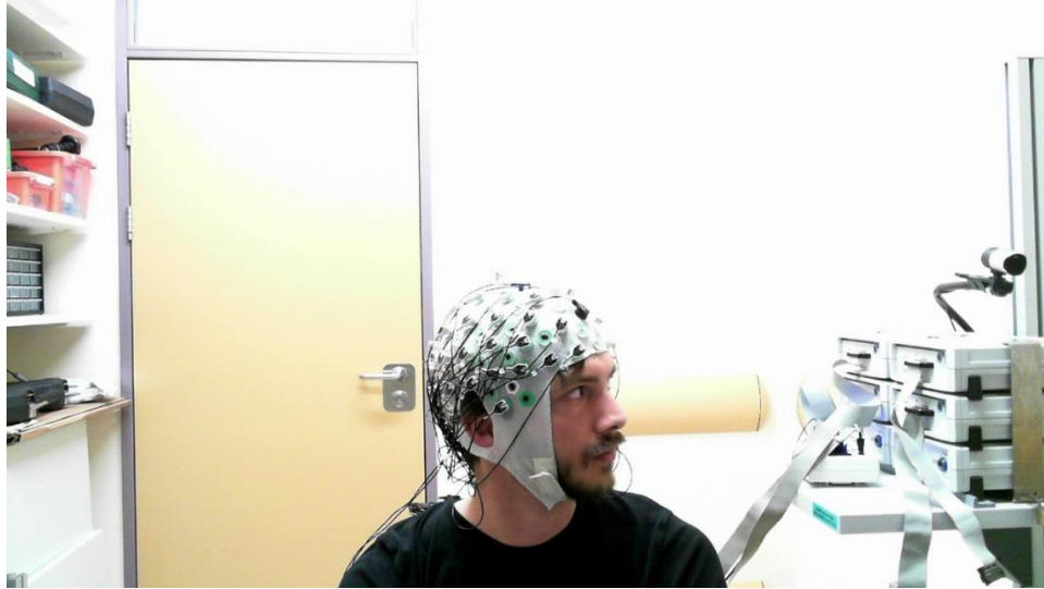
Figure 6 Picture taken during a pilot study, showing the subject station and one of the 32 electrodes EEG setup in use at our laboratory (Picture courtesy of Maja Kapitler and Filip Agatić).
