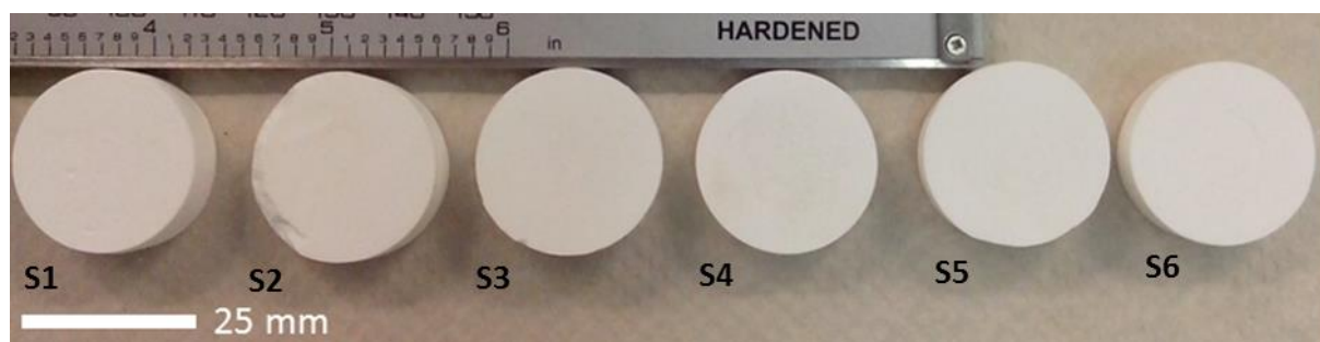
Figure 4-10. Photographs of polyMIPE samples for compression test produced by polymerisation of emulsion templates E20-60. A smooth surface was visible after polishing. The sample S2 was discarded because of surface defects.
