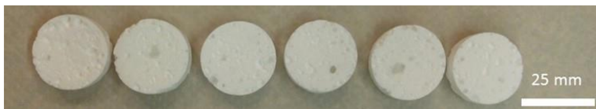
Figure 4-9. Compression test samples synthesised from emulsion templates E10-60. The internal pore structure contained a few large pores with a size between 3-6 mm.
