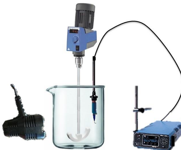
Figure 5-2. Schematic of the setup used for the production of beads by “in suspension” polymerisation.
