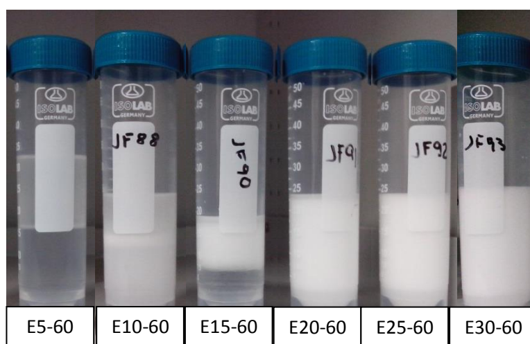
Figure 4-2. Photographs of emulsions with an internal phase volume ratio of 60 % stabilised by different surfactant concentrations. From left to right, the first three emulsions were stabilised by 5, 10 and 15 vol.% of surfactant and phase separated after a few minutes. The last three were stabilised using 20, 25 and 30 vol.% of surfactant. No signs of phase separation were visible after one week.
