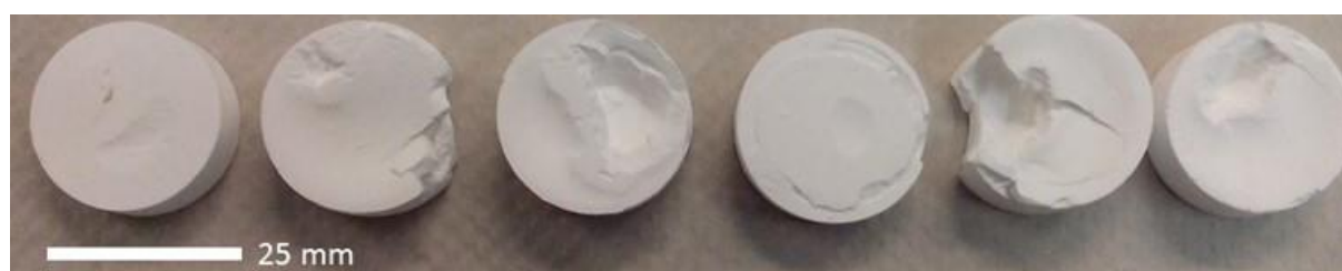
Figure 4-12. Monoliths produced by polymerisation of emulsion templates E30-60. Only a polymerised layer between 3 - 4 mm was formed after UV irradiation for approximately 20 min. All samples were discarded.
