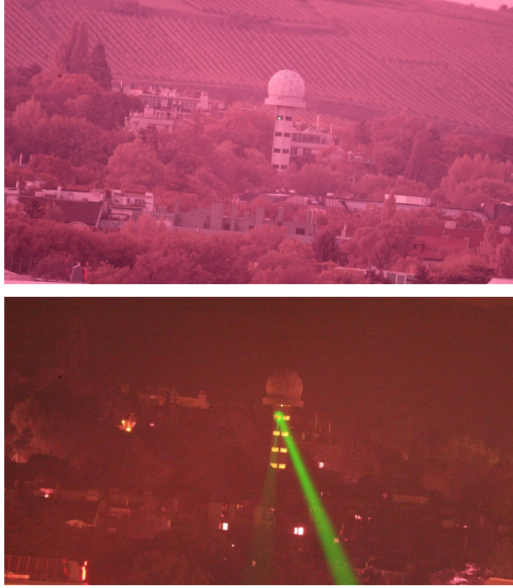
Figure 4.3: Image of the sending station at the radio tower at ZAMG. The upper image is taken during the day, the lower image is recorded during the night. In the lower image, there are two lasers visible: A faint green laser beam which is sent from the ZAMG tower to the receiver (difficult to see, on the left of the strong green laser), and a strong green laser beam which is used as alignment laser from the IQOQI Vienna building to the ZAMG tower. The strong laser can also be seen in figure 4.1 in the top image.
