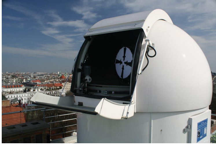
Figure 4.11: A picture of the Hedy Lamarr Quantum Communication Telescope at the roof top of the IQOQI building, with the absorptive mask for \ell = \pm 2
