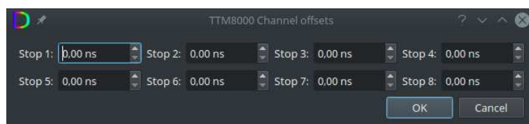
Figure 1.2 Managing the delay offsets per channel for counting coincidences with the TTM8000.
