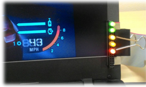
Figure 13. – Five LED Stripe used for an attention level visual feedback to the gamer
