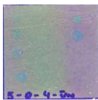
Figure 52: Inconel – 20% w/v PLGA – 0.1% v/v Desmodur®; after 4 h incubation at 4°C
