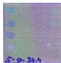
Figure 53: Inconel – 20% w/v PLGA – 0.1% v/v Desmodur®; after 4 h incubation at 37°C
