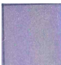
Figure 57: Inconel – 25% w/v PLGA – 1% v/v Desmodur® + 0.25% w/v Carmin red; before incubation
